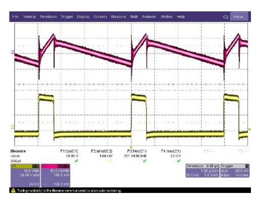
Figure 12. Vin = 24 V, Vout = 3.3 V, lout = 1.5 A, C1 = Vout, C2 = VSW
