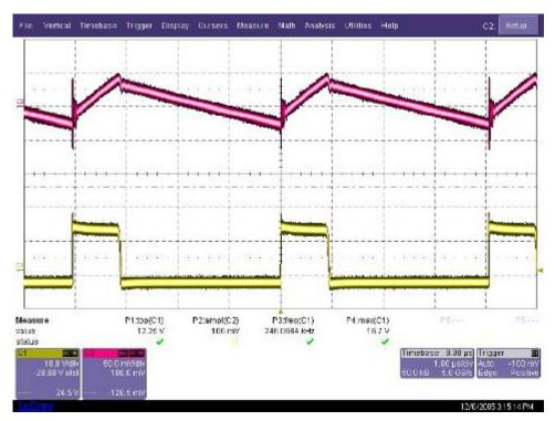
Figure 19. Vin = 18 V, Vout = 3.3 V, lout = 1.5 A, C1 = Vout, C2 = VSW
