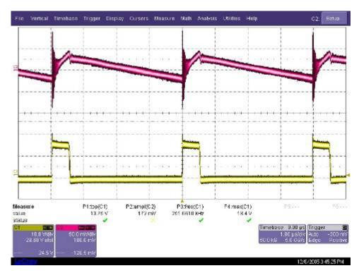
Figure 16. Vin = 18 V, Vout = 1.8 V, lout = 1.5 A, C1 = Vout, C2 = VSW
