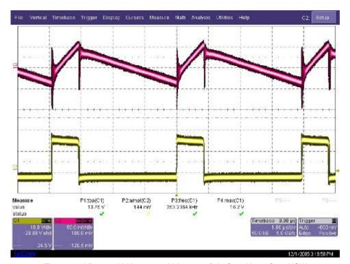
Figure 11. Vin = 18 V, Vout = 3.3 V, lout = 1.5 A, C1 = Vout, C2 = VSW
